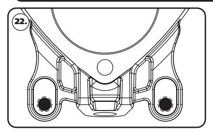
**22.** The threaded steering arm inserts can be mounted in 2 different positions. **Image 22** illustrates the correct position for the installation on your vehicle. This position is what we determined to be the best with Ridetech suspension.
