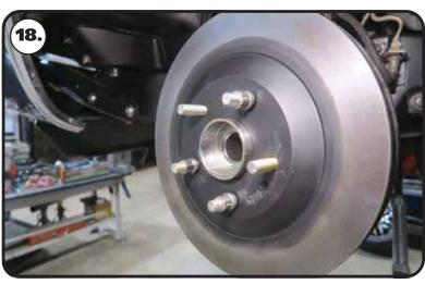
**18.** Install the rotor on the hub. Thread some lug nuts on the threads of the hub to hold the rotor tight on the hub.
