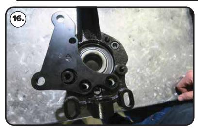
**16.** The caliper brackets are side specific. They have a D & P stamped in them. Lay the correct side caliper bracket on top of the shims, aligning the mounting holes with the mounting holes of the bracket. The counter sunk holes should facing up.
