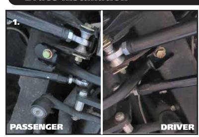
**5.** The new suspension brace bolts in place of the original brace. Install a 1/2" split lock washer & 1/2" flat washer on each of (2) 1/2"-13 x 1" bolt. Position the crossmember brace at the factory location, behind the lower control arm mount. Align the mounting holes of the crossmember with the mounting holes in the frame rails. Install a bolt/washer in each of the mounting holes. Torque the crossmember hardware to 50 ftlbs.
