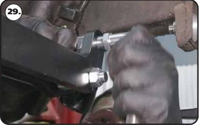
**29.** The studs with the short hex get installed into the centerlink adapter. The short side goes into the adapter attached with the 5/8"-18 thin top lock nut, with the long side of the stud pointing forward.
