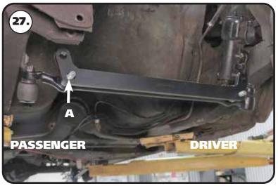
**27.** The centerlink bracket has one attachment hole [A] that is slotted. This is to accommodate the variations in manufacturing and machining processes, as well as any wear that may have occurred to the original centerlink over time. The slot goes on the passenger side centerlink adapter stud.
