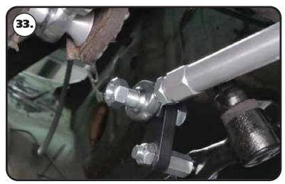
**33.** Install one end of the tie rod onto the stud of the centerlink adapter. Install a 5/8"-18 mechanical locking nut on the threads of the stud and torque to 45 ftlbs.
