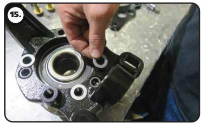
**15.** Lay a .062" thick, 1/2" ID shim on each of the caliper brackets (3) mounting holes.
