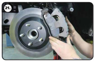
**21.** Install the brake pads and caliper.
