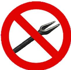
NEVER USE A "WEDGE" OR "PICKLE FORK" TO SEPARATE SUSPENSION OR STEERING PARTS YOU INTEND TO RE-USE. ALWAYS USE THE PROPER PULLER FOR THE JOB TO AVOID DAMAGE.
